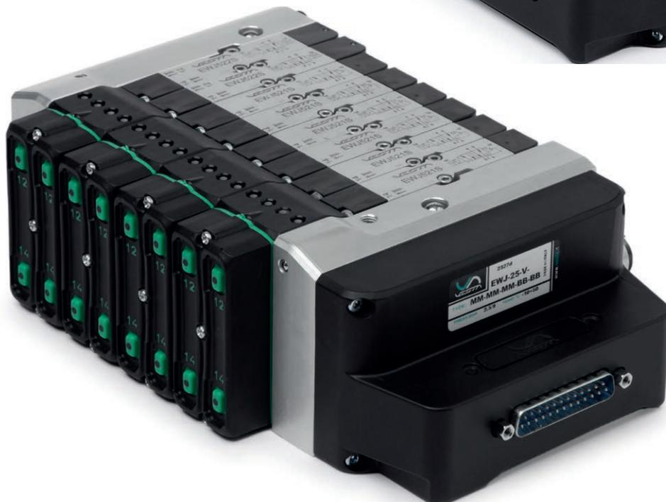
All valve combinations available: 5/2, 5/3 and double 3/2 valve. All valves can be single or double solenoid, easy to assemble and quick to change even when the system is already mounted. A single assembly can have as many different pressure values as needed, by using intermediate separators and air supply on both end plates. Due to EWJ electronics, no solenoid stations are ever wasted.
